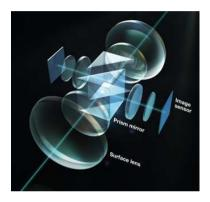
Solution for small shape: Inflection optical method (deflect incident light and guide it to the image sensor)
